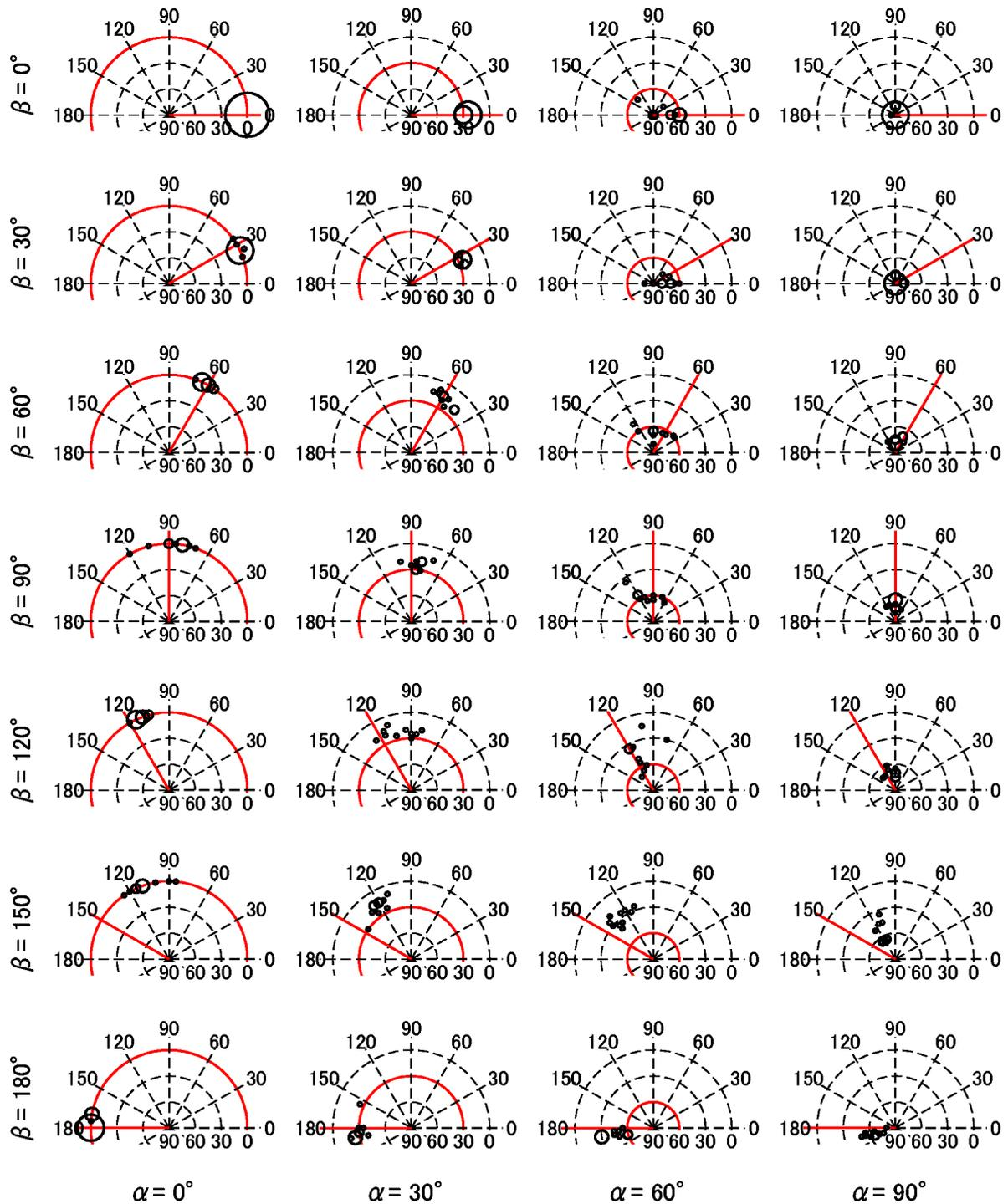
Figure 2. Responses to the stimuli, which simulated ITD, ILD as interaural differences. The circular arcs denote the lateral angle  $\alpha$ , and the straight lines denote the vertical angle  $\beta$ . The simulated lateral angle and vertical angle are shown in bold lines.
