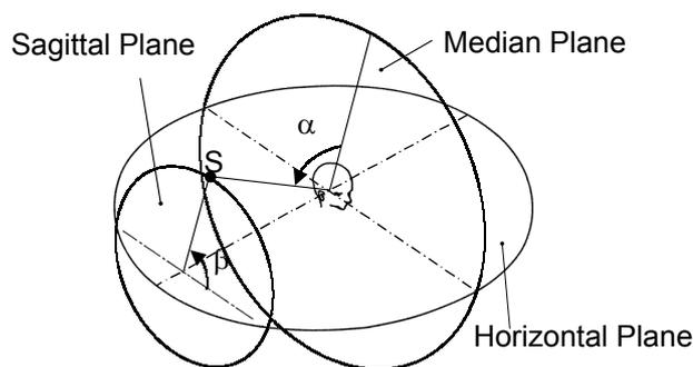
Figure 1. Definition of the coordinate system.  $\alpha$  is the lateral angle and  $\beta$  is the vertical angle of a sound source,  $S$ .
