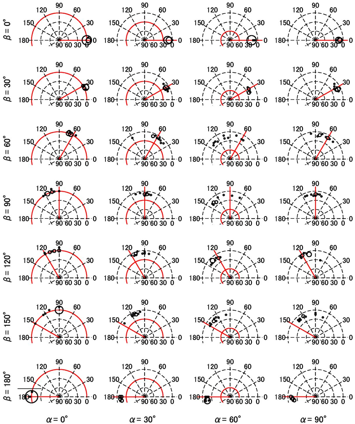
Figure 4. Responses to the stimuli, which simulated only ILD as interaural difference. The circular arcs denote the lateral angle  $\alpha$ , and the straight lines denote the vertical angle  $\beta$ .
