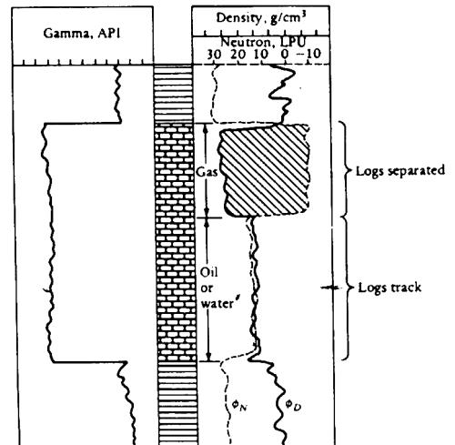
Figure 1: Radiation logs in a reservoir [17]
