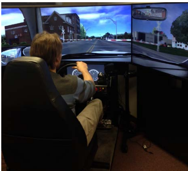
Figure 1. NADS MiniSim simulator as a research platform
