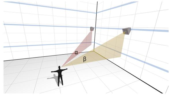
Figure 6: In a layered approach, depending on the architecture, loudspeakers within the same layer may have slight angle anomalies from the perceiver's vantage point, as is the case here with angles  $\alpha$  and  $\beta$ .
