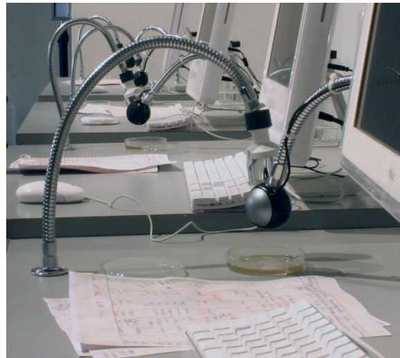
Figure 3: Web camera focused on a Petri-dish with sample of Daphnia .
