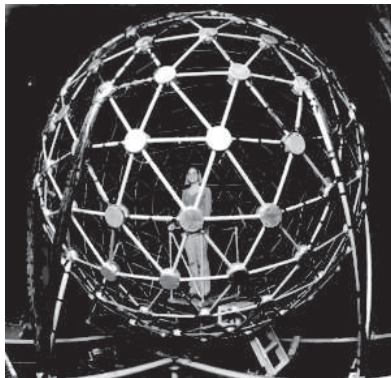
Figure 1: Auditory Localization Facility used for HRTF collection
