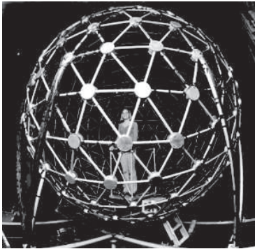
Figure 1: Auditory Localization Facility used for HRTF collection
