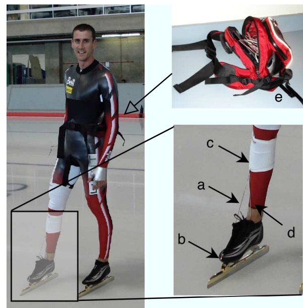
Figure 4: The sensor installed on the model skater: The variable-resistance elastic (a) is connected between a skate lace near the toe (b) and an elastic joint-support band (c) (used only to fasten the sensor). In this configuration, R_s (and therefore the voltage measured by the interface kit) increases with ankle extension. Leads (d) connect the sensor to the phidget interface kit ( http://www.phidgets.com ) and netbook computer worn by the skater in a waist pack (e). Sound is broadcast through headphones (not shown).
