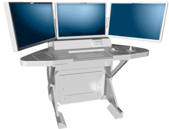
Figure 1: Three-screen console configuration of the Common Display System, the new information workstation being acquired for the U.S. Navy’s modernization program and next-generation surface ships.
