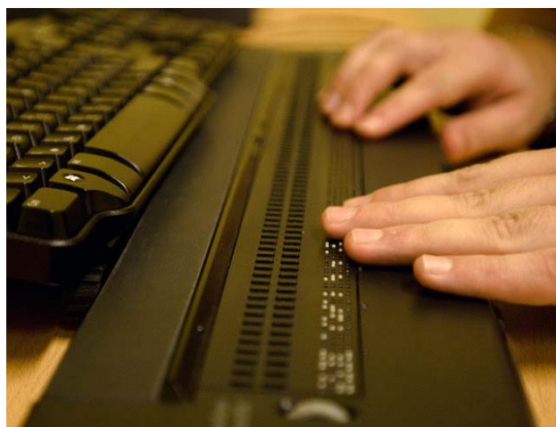
Figure 2. The Braille input/output module [14].
