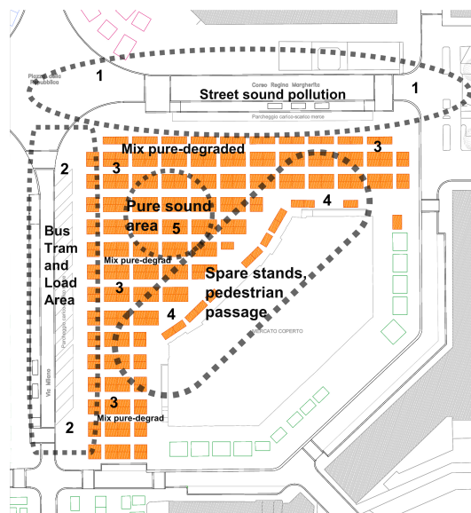
Figure 7: Map of a portion of the Balón market: numbers and names indicate sound zones identified during the annotation phase.
