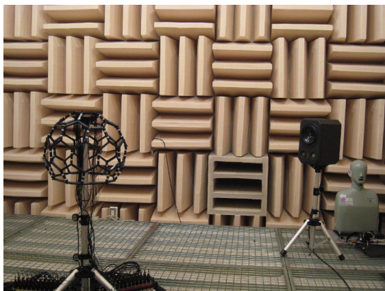
Figure 9: Experimental setup. Impulse responses between sound source and C80 microphone array are measured in an anechoic room.
