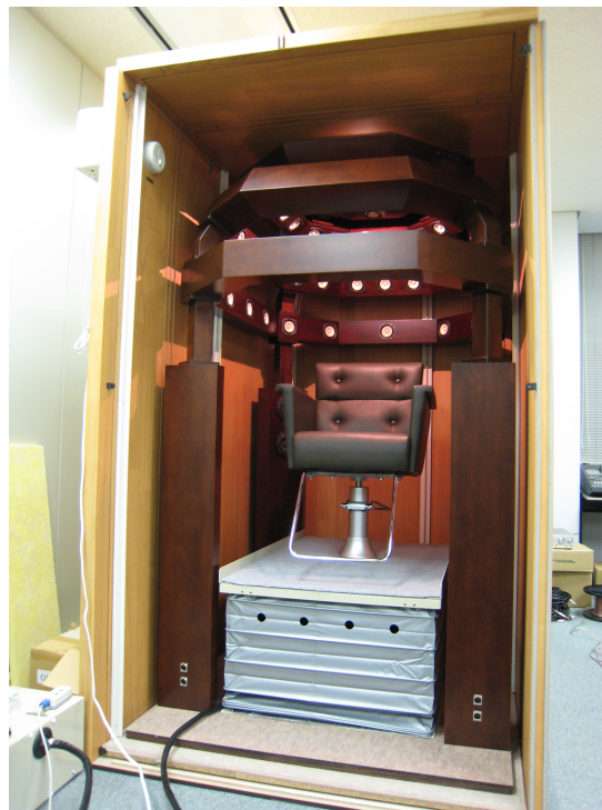
Figure 3: 3D sound field reproduction room. This room is constructed using a sound-proofed room to reduce the noise. The loudspeaker system, a hydraulic lift and a chair are installed in the room. The hydraulic lift and the chair raise the user's head into the 3D sound field reproduced area.
