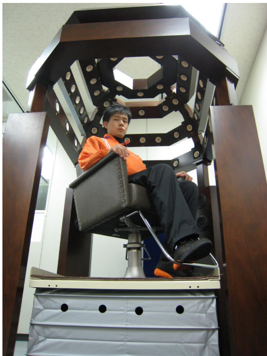
Figure 2: Loudspeaker system to reconstruct a 3D sound field recorded by a C80 fullerene-structured microphone array that consists of a dome structure and a support pillar. The dome structure part has four mounting racks and six full-range units, and 16, 24, and 16 units are installed on them, respectively.
