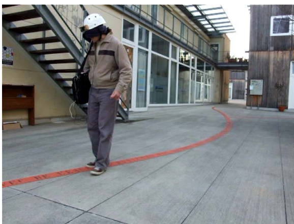
Figure 3. A blindfolded individual following a colored line with a head mounted webcam and a notebook carried in a shoulder pack.
