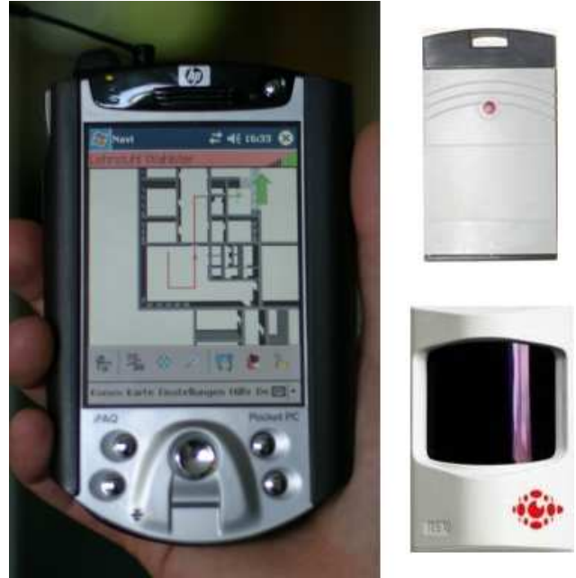
Figure 3: iPAQ with active RFID reader installed, an RFID tag and an infrared beacon.
