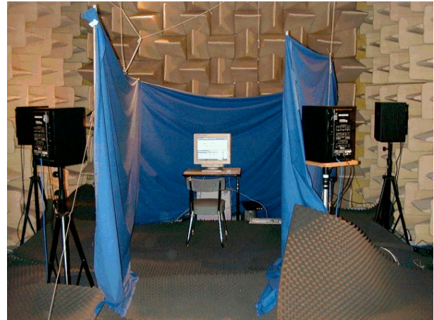
Figure 2. Reproduction set-up where the six loudspeakers are hidden behind acoustically transparent curtains.
