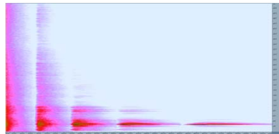
Figure 7. Spectrographic view of a room impulse response auto-convolution sequence. The original impulse response is on the left, followed by progressive auto-convolutions. The frequency scale (vertical) is 0-5 kHz (linear), and the time scale duration is 15 s.
