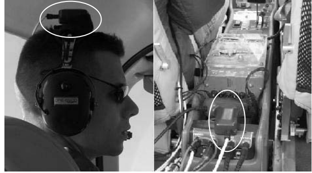
Figure 2: Configuration of orientation tracking device in the head-slaved (left panel) and plane-slaved (right panel) conditions of the experiment. In each case, the location of the IMU unit has been circled.
