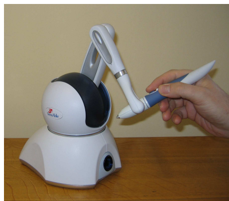
Figure 1: A picture of a SensAble Technologies’ PHANTOM Omni Haptic Device. The use of motors and optical sensors allows the user to “feel” virtual objects.
