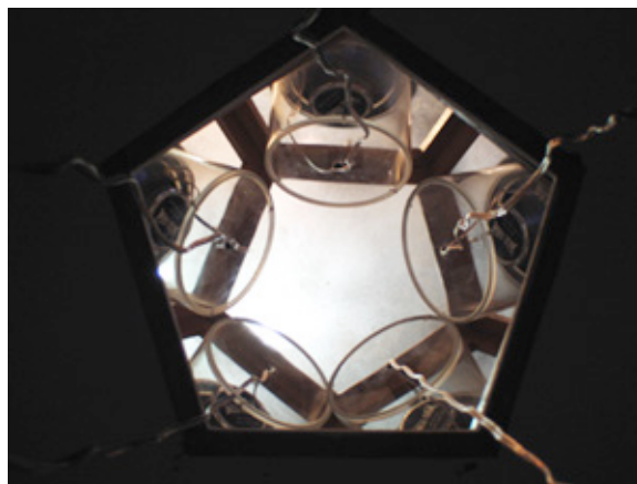
Figure 2 shows five of the ten loudspeakers each positioned in the centre of one of the pentagons on the side of the structure. An image projector is mounted in the plinth and projects through the pentagon at the base of the structure onto the pentagon at the top.
