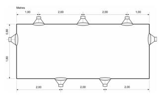
Figure 3. Loudspeaker placement on DigiWall
