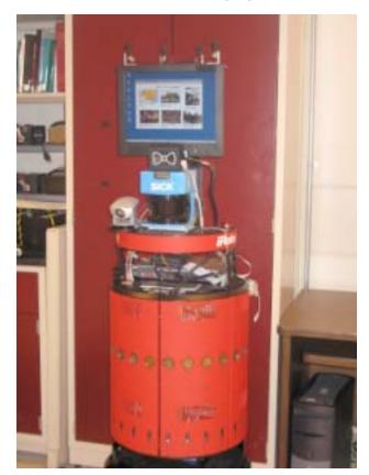
Figure 1. A mobile iRobot B21R configured with microphones, an amplified loudspeaker, and a visual display to function as an information kiosk.
