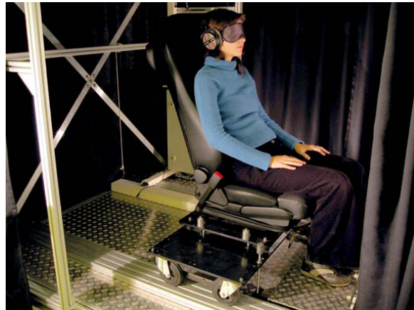
Figure 2. Laboratory setup: a participant sitting on a chair mounted on a wheeled platform coupled with a footrest.
