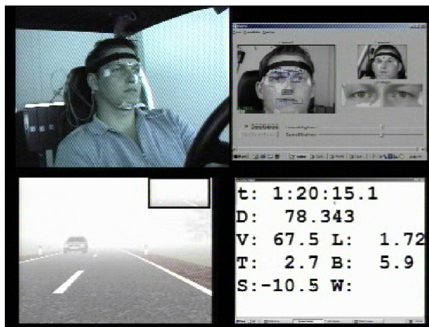
Figure 1. Split-screen picture showing the subject (top left), the driving scene (bottom left), the faceLAB-screen (top right) and the current driving parameters (bottom right).
