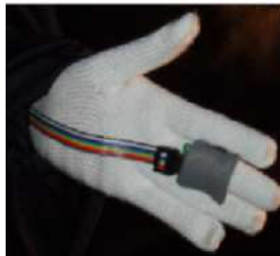
Figure 1: 3-D accelerometer used to sense movement
