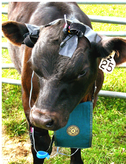
Figure 9. Sensor-Cow: bi-directional (mercury) motion sensors are attached to the calf's front legs, a gyroscopic sensor on the forehead and accelerometer on his right ear. The pouch hanging around his neck contains the radio frequency transmitter that sends the real time data to the (La Kitchen) Kroonde Gamma wireless UDP receiver [23]. It is connected by Ethernet to the computer running the data sonification with Max/MSP object-oriented programming environment.
