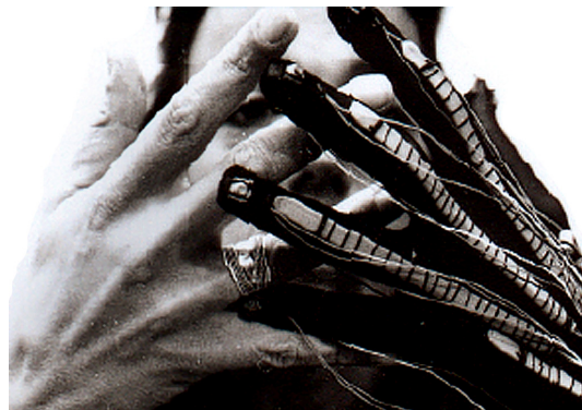
Figure 8. A gestural Cyberglove controller that produces a high degree of accuracy transmitting spatial, position, rotational, gyroscopic, velocity and flex data. The precision facilitates interaction with information representation in 3D space [22].
