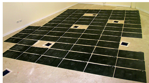
Figure 5. The author's Sensate Lab (2 views) showing the "invisible" pressure sensitive floor mats embedded underneath the carpet, triggering the visual and auditory sound system and (before carpeting) the grid of pressure mats, networked to the Telio modules.
