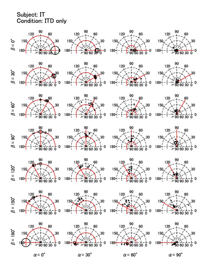
Figure 3. Responses to the stimuli, which simulated only ITD as interaural difference. The circular arcs denote the lateral angle  $\alpha$ , and the straight lines denote the vertical angle  $\beta$ .
