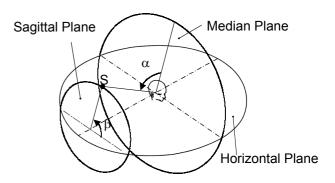
Figure 1. Definition of the coordinate system.  $\alpha$  is the lateral angle and  $\beta$  is the vertical angle of a sound source, S.
