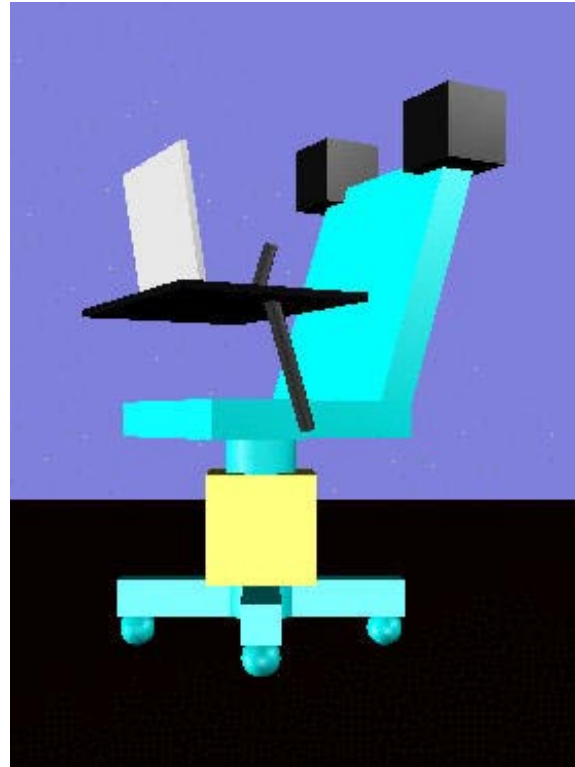
Figure 16: Internet Chair with servomotor rotation: a pivot (swivel, rotating) chair deployed as an I/O device, an information appliance. The input modality is orientation tracking, which can dynamically select transfer functions used to spatialize audio in a rotation-invariant soundscape. In groupware situations, like teleconferencing or chat spaces, such orientation tracking can also be used to twist iconic representations of a seated user, avatars in a virtual world, enabling social situation awareness via coupled visual displays, soundscape-stabilized virtual source locations, and direction-dependent projection of non-omnidirectional sources. As an audio output modality, transaural speakers (without crosstalk), nearphones in the headrest, can present unencumbered binaural sound with soundscape stabilization for multichannel sound image localization. As a haptic output modality, servomotors will render kinesthetic force-feedback, turning each chaire (pronounced “schaire,” for “share-chair”) under networked control, distributing torque across the internet to direct the attention seated subjects (with adjustable insistence/forcefulness), orienting seated users (like a “dark ride” amusement park attraction), or subtly nudging them in a particular direction. (Java3D model by Daisuke Kaneko; 金子 大輔.)
