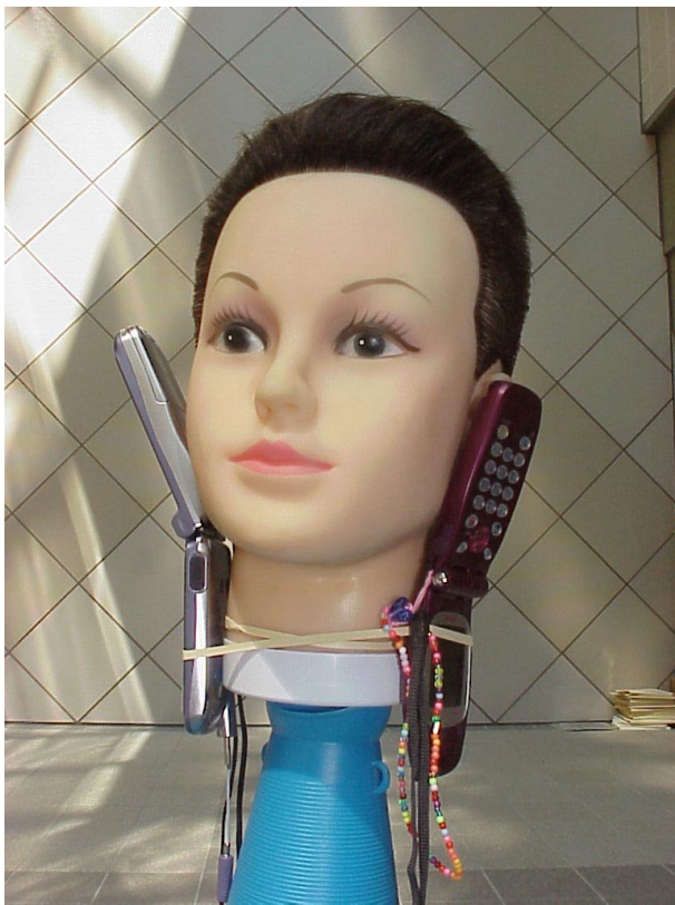
Figure 7: “Poor person’s mobile stereotelephony”: a pair of inverted mobile phones, deployed as a microphone array attached to a dummy head, simultaneously calling a dual voice line (like an ISDN service) realizes wireless (if low-fidelity) binaural telepresence.
