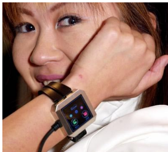
Figure 14: NTT DoCoMo “Whisper Wearable Terminal.” By sticking her finger in her ear, a user can hear sound conducted through arm, hand, and finger bones while speaking into a microphone on the back of the wristband, snapping fingers to signal “connect” and “disconnect” commands. The manufacturer hopes to release a commercial model in 2005. Presumably a stereotelephonic system could be realized by sticking fingers in both ears.
