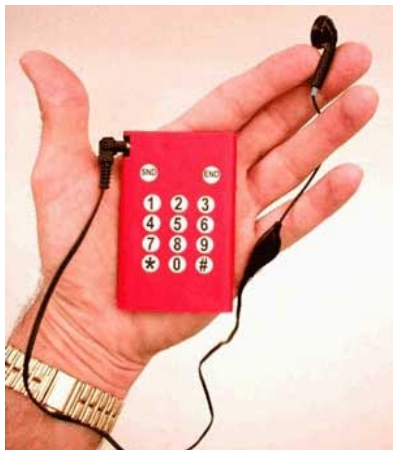
Figure 10: Dieceland Technology disposable mobile phone ( www.dtcproducts.com ): This 2" x 3" (the size of a thick credit card) disposable ($10) mobile phone is made by printing cell-phone circuitry onto a paper substrate, which is then laminated.
