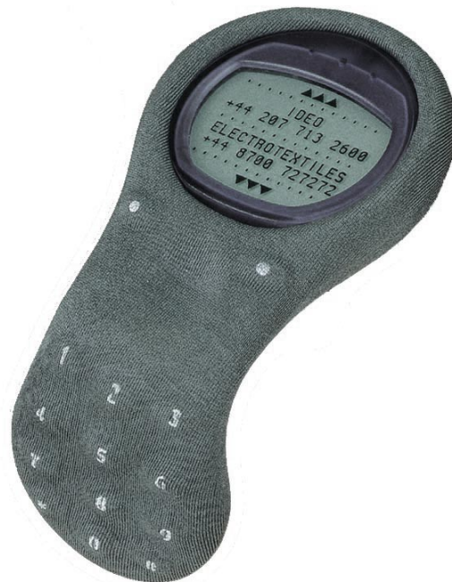
Figure 9: ElekTex soft cell phone ( www.elektex.com ), with touch controls integrated into the fabric. (©ElekSen. Photo by Marcus Rose.)
