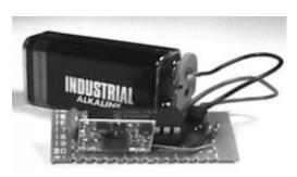
Figure 1: Left - The inside of the wearable device showing the Diamond  $\operatorname{Rio}^{TM}$ , the RF receiver, the PIC microcontroller and a 9V battery. The inset is the closed unit. **Right** - The RF transmitter attached to a 9V battery.
