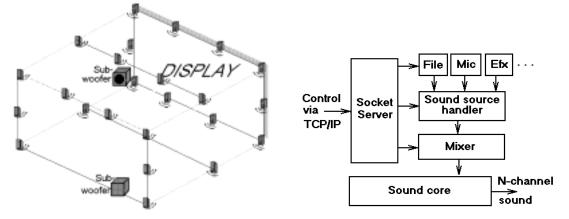
FIGURE 1. 26 Speaker array in Video Wall room.
