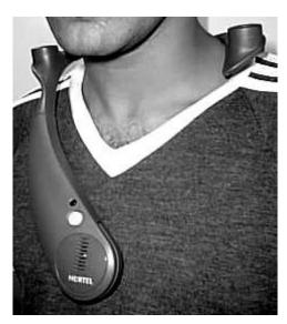
Figure 2: The wearable audio device, the Soundbeam, with directional speakers and microphone
